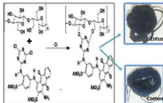
Fig. 6: Reactive dye interaction mechanism with Lotus fibres.
